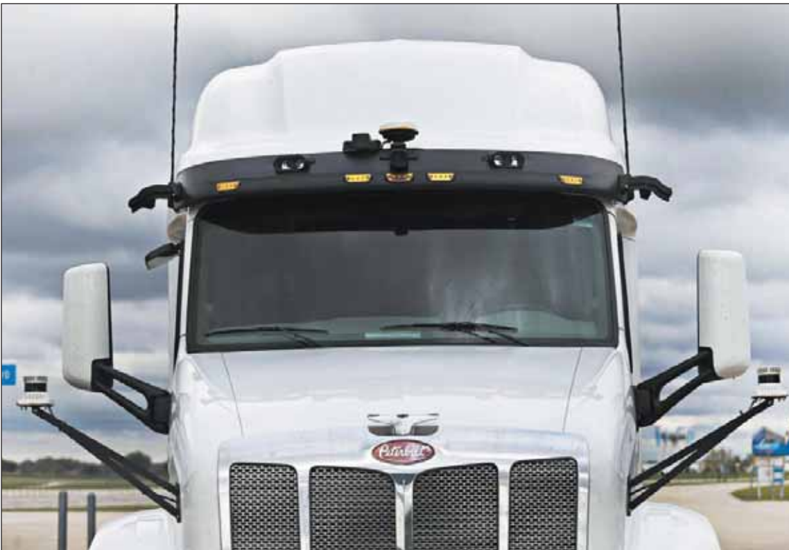
The Autobon wind visor is equipped with cameras, sensors and an acceleration meter.
