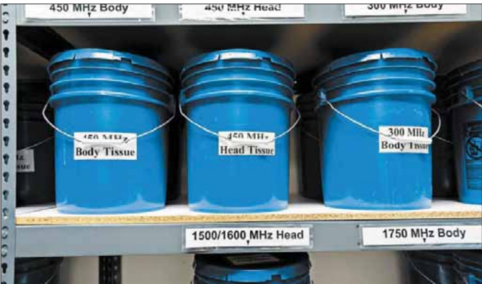
RF Exposure Labs uses different liquids to simulate the electrical properties of human tissue.
