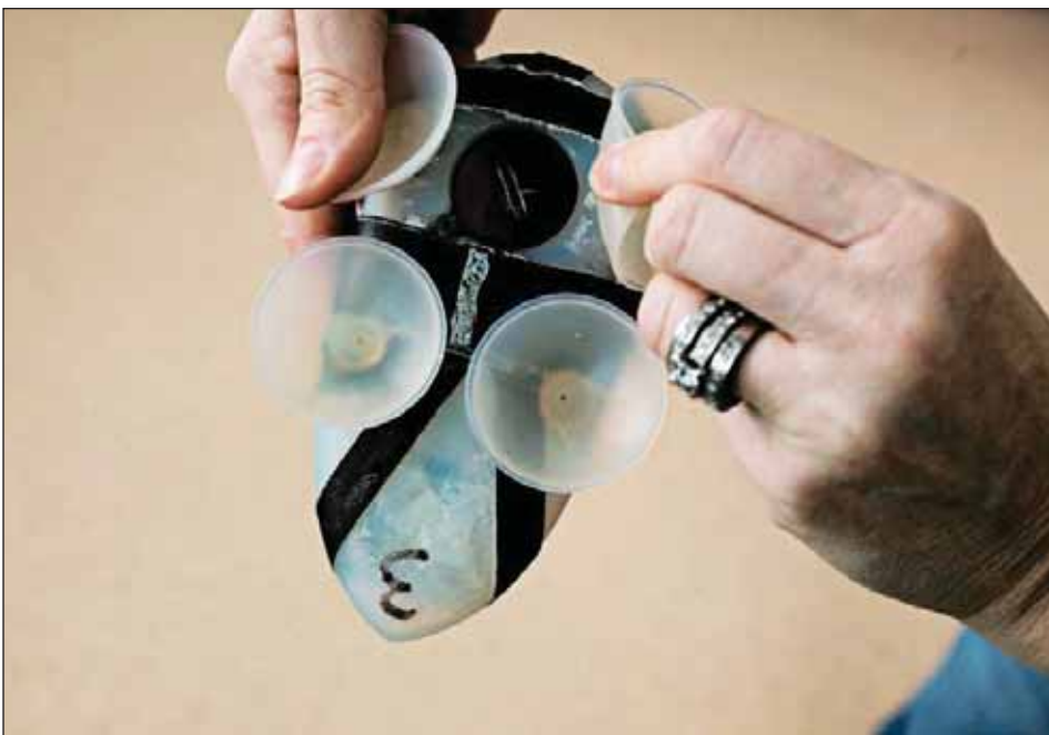
The MTag, or Movement Tag, is a motion-sensing data logger that records acceleration, speed, angular rate, temperature and depth.
